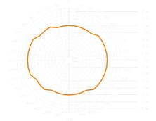
Presence Control PRO HF 360 installation height 2.8 m (orange = radial)
